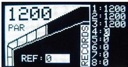
The system then displays the « **RECORD** » screen, which allows you to record 8 different measurements. These measurements remain saved even when the device is turned off or when the battery is changed.
